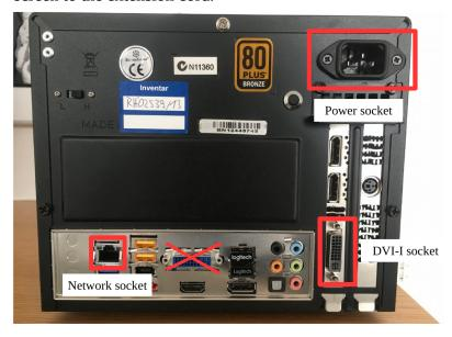
3. Turn on the workstation and the screen. Select display channel "HDML 2". The login screen should appear.
